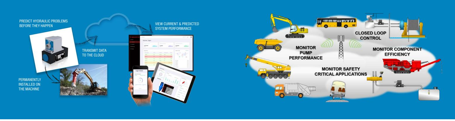
So the performance level of pumps and actuators can most easily be determined by monitoring their output or input flow using a simple, robust flow monitor permanently installed in the system. Such a unit is the Webtec CTA series turbine type flow monitor which provides both a temperature and a flow rate output signal compatible with SAE J1939 CANbus communication as used on many vehicles.
