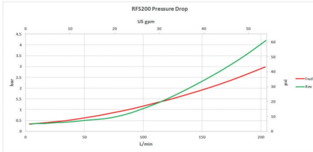
Typical pressure drop with 1" BSPP fittings. 1 bar = 14.5 psi, [ISO32 @23cSt]
